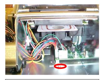
Connect all cables, remove adhesive liner and attach controller bracket to bottom of printer, behind post, as shown
