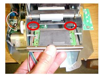
Slide encoder bracket into position and spacer bracket is engaged into mounting holes. Ensure bracket feet are resting on top of side rails. Secure spacer bar screws.
